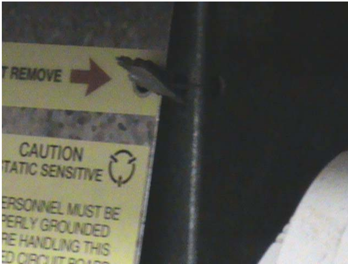
Figure 2: Serial-numbered crimped metal CPU security seal
