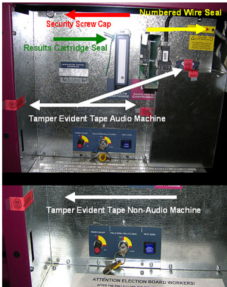
Figure 3: New Jersey's instructions for proper sealing of the AVC Advantage.
